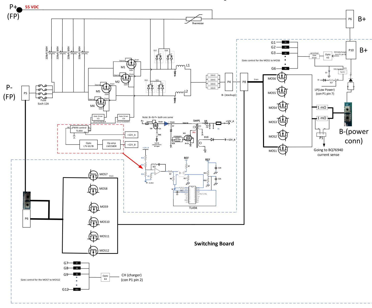
TI: I assume B+ and B- are your 48V output terminals. But your circuit shows TL494 feedback from +12V\_A, which is to use TL494 to regulate +12V\_A. But I cannot find how 48V (B+ and B-) is regulated from +12V\_A. Can you describe how 48V is regulated by TL494?
