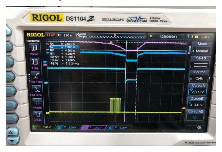
Trace 1 (Yellow) is the output to the MEMS switch from the MCU.
