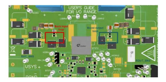
For both input and output current sensing resistors, differential sensing and routing method are suggested and highlighted in the Image below. Use wide trace for gate drive traces, minimum 20 mil trace width. Connect all analog grounds to a dedicated low-impedance copper plane, which is tied to the power ground underneath the IC exposed pad.
