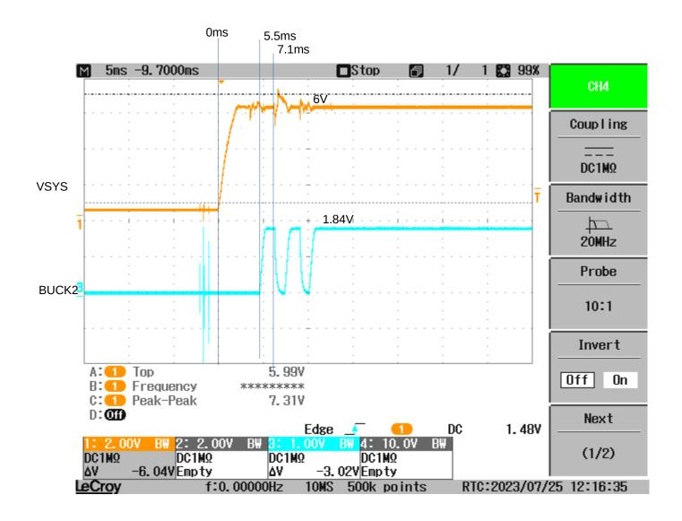
Voltage at  $500m\Omega$  load is 0.85V. Voltage at BUCK2 output is ~1.8V
