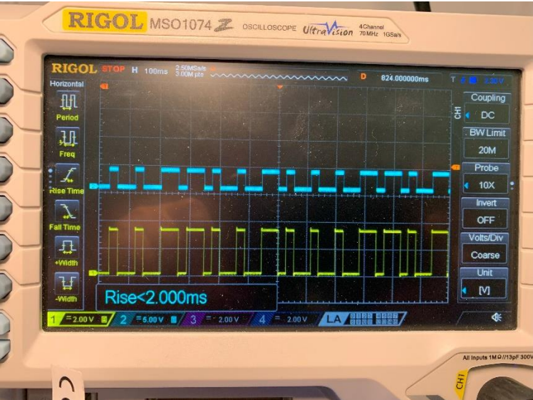
Just USB-C Cable Attached – showing CC lines TI TPS25751EVM
