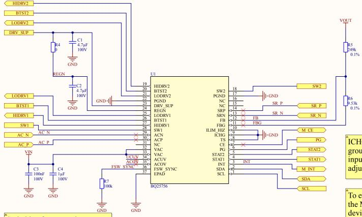
ICHG and ILIM\_HIZ are shorted to ground for disabling hardware limit for input and charge currents. These can be adjusted through the registers.
