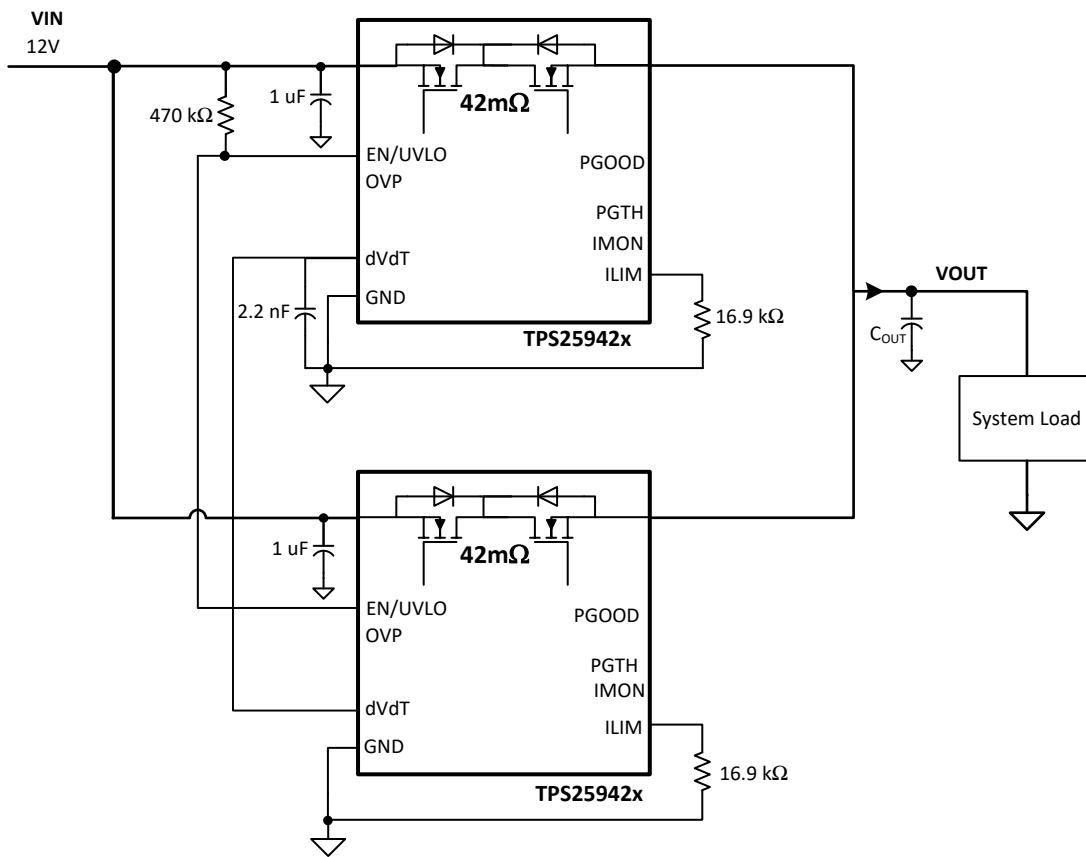
**Circuit Configuration for Parallel Operation of two eFuses**
