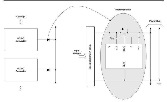
Figure 1. Redundant System Using TPS2412 OR-ing FET Controller
