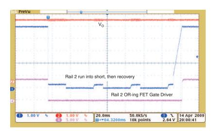
Figure 5. Rail 2 Run Into Shorted Then Recovery
