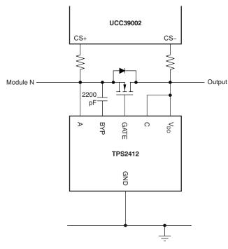
Figure 6. OR-ing FET  $R_{DS,On}$  Used for Share Current Sensing
