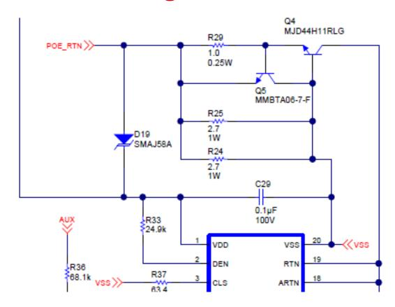
The current booster circuit TI uses is current based and turns on when more current is needed by the system. This makes the design more robust and accurate
