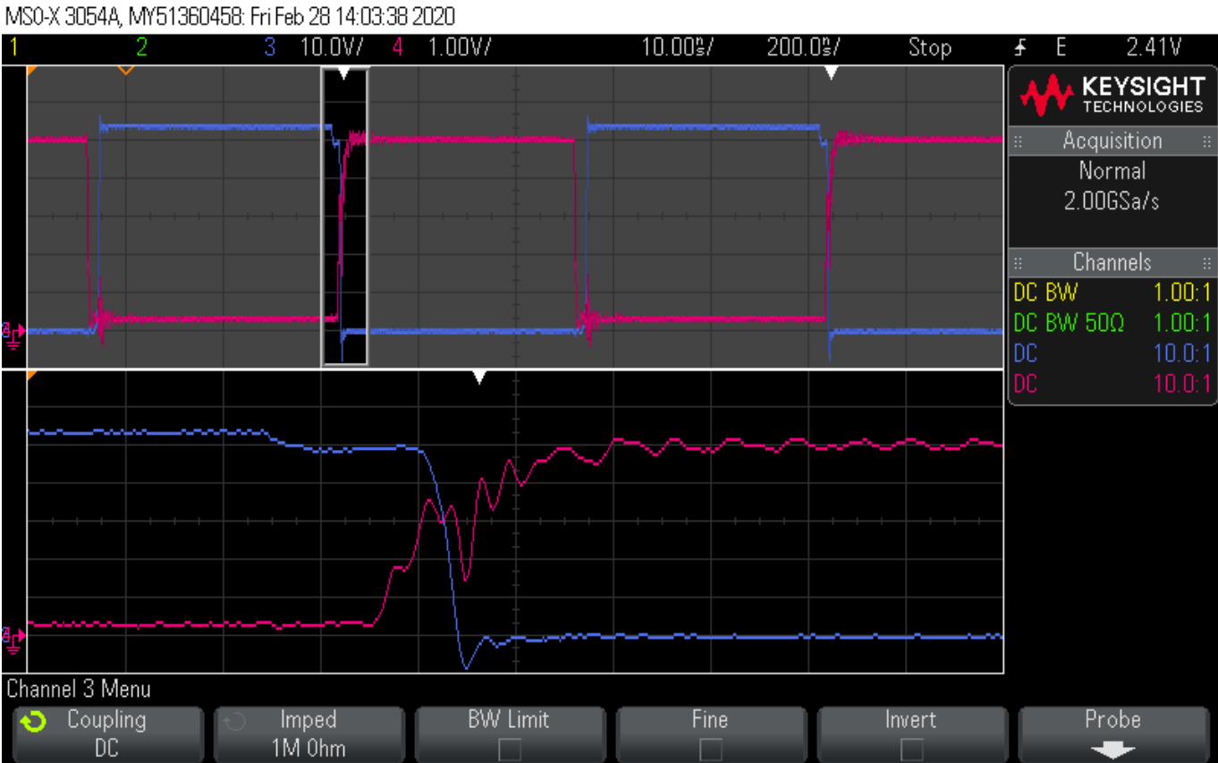
Figure 4 - HO and LO during HS falling, 10nS DT
