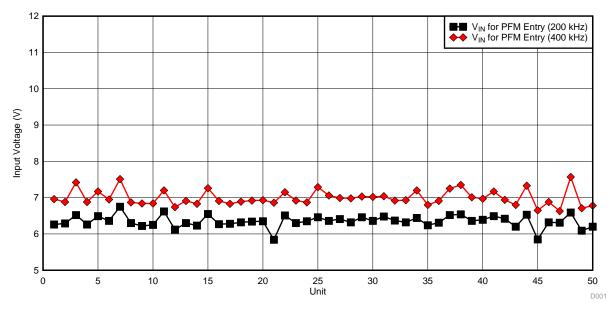
As for comparison, below is the test result for 50 units of the LM43603A-Q1 version
