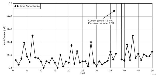
Figure 3. LM43603-Q1 Input Current at 8.5 V<sup>IN</sup> and 5 V<sub>out</sub> With 0.5-mA Standby Load
