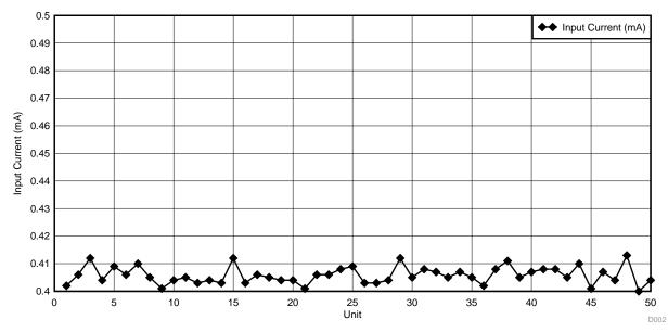
Figure 4. LM43603A-Q1 Input current at 8.5 V<sub>IN</sub> and 5 V<sub>OUT</sub> with 0.5-mA Standby load
