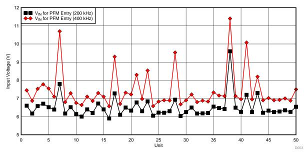
Figure 1. LM43603-Q1 PFM Entry Input Voltage for 5-V Output With 12.2-µH Inductor and 0.5-mA Standby Load
