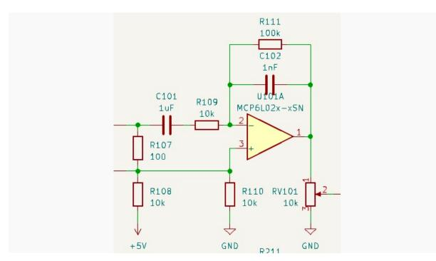
This is a band pass filter with following characteristics:
