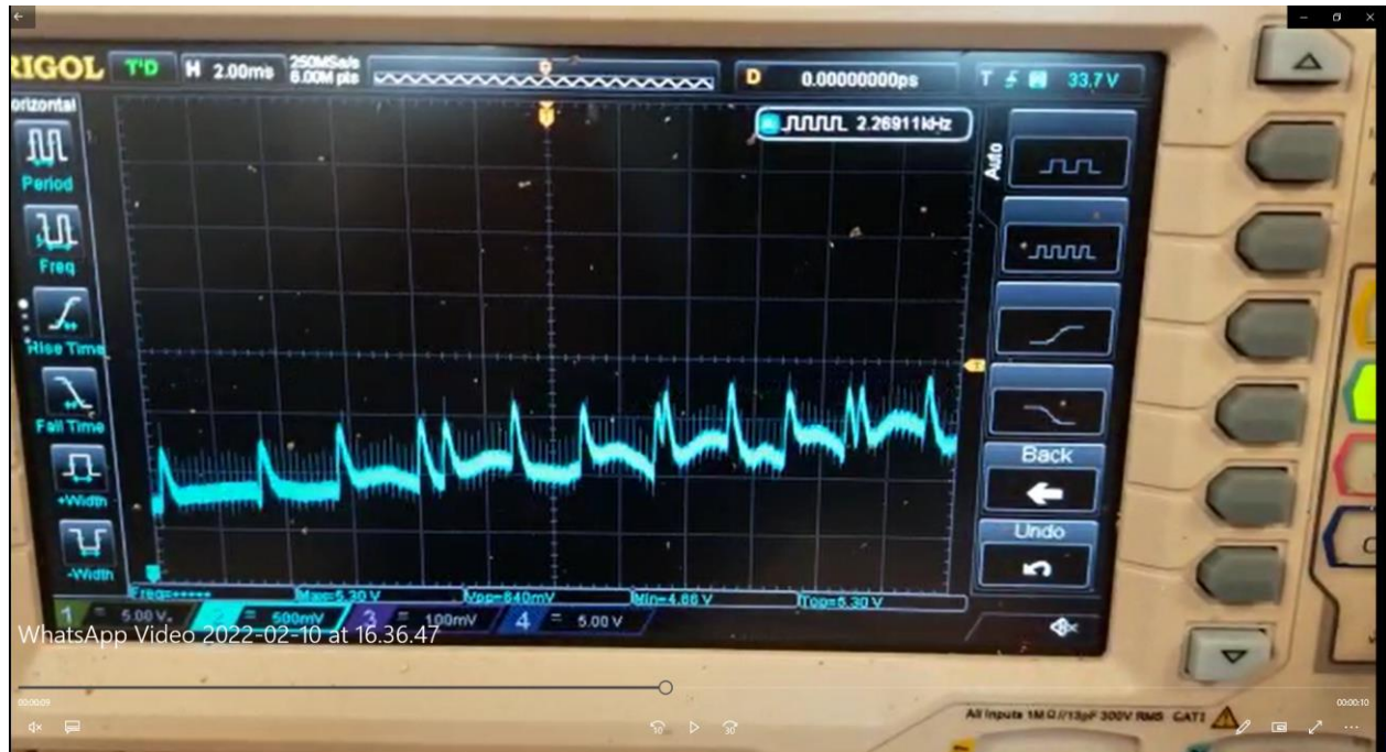
Figure 10: Waveform during transition from move forward to move backward. V_{max}=5.3 V_{min}=2.92V (although the screen shows around 4.7V, The 2.92 V appears for very short time)
