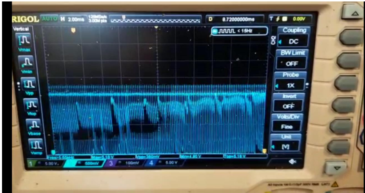
Figure 4: Waveform captured during transition from go forward to go right command.
