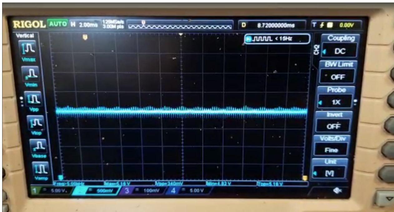
Figure 5: Waveform captured during go right command. Vpp=340mV, Vmin=4.82V and V max = 5.16V.
