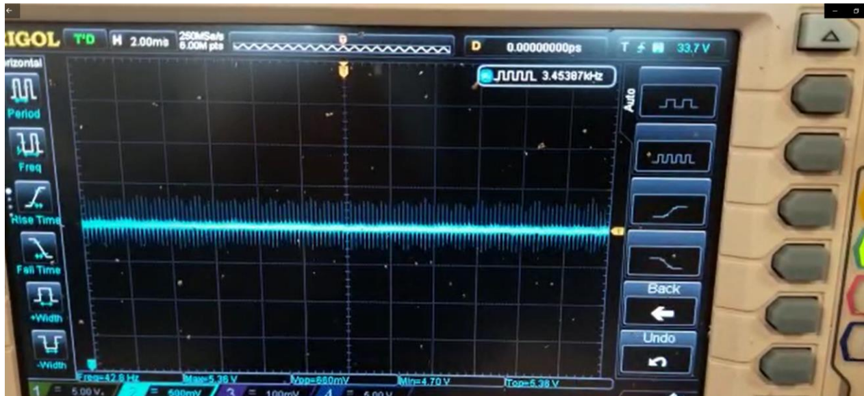
Figure 11: Waveform captured on 5V line, (normal operation move backward or move forward, both motor are on with full speed). V_{pp}=600\text{mV} , V_{min}=4.7\text{V} and V_{max}=5.3\text{V}
