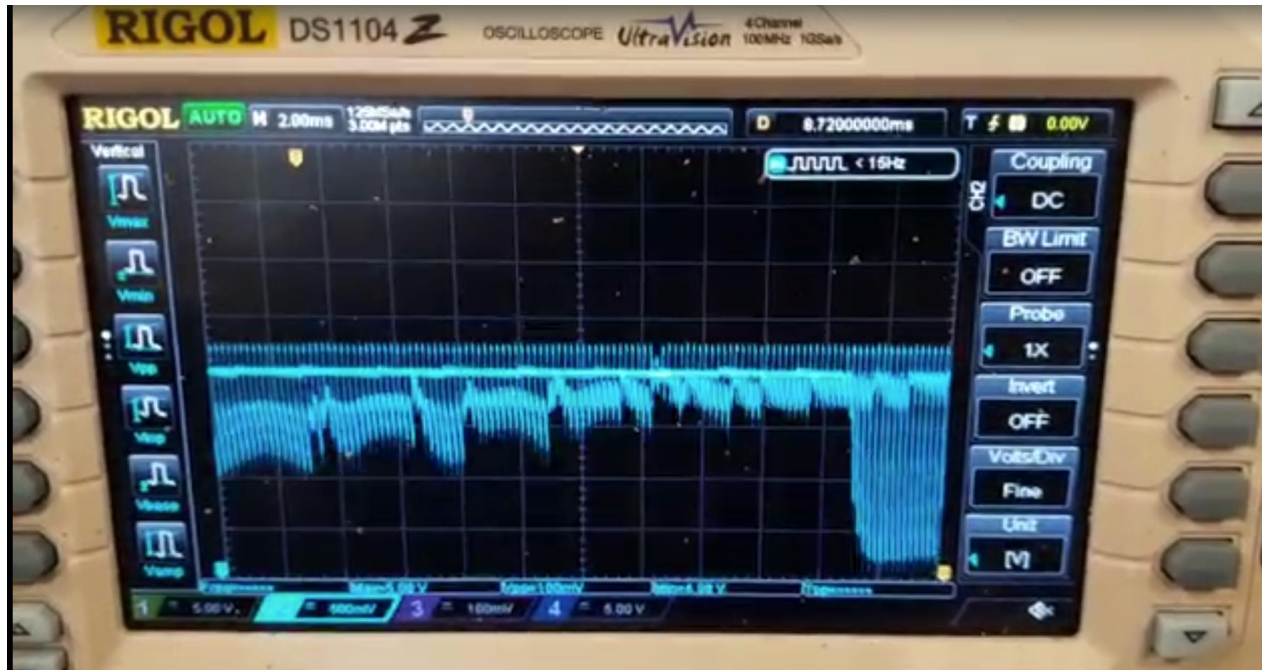
Figure 2: Waveform captured during first startup of the PCB with two motors connected
