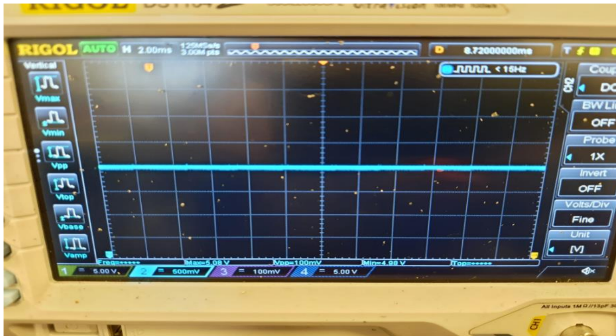
Figure 1: 5V output when motors are not connected. Vpp of ripple was 100mV, Vmax 5.08V and Vmin=4.98V
