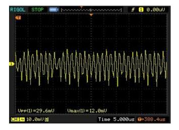
+15V dynamic response (25%~75% load (15V/200mA), 100Hz frequency):
