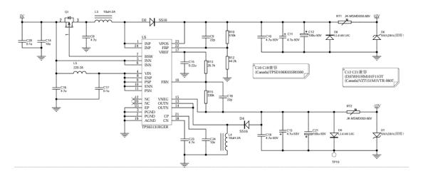
Actual test circuit with C18, C9 in series with 51K resistor; C18 to  $100 \text{pF}_{\circ}$
