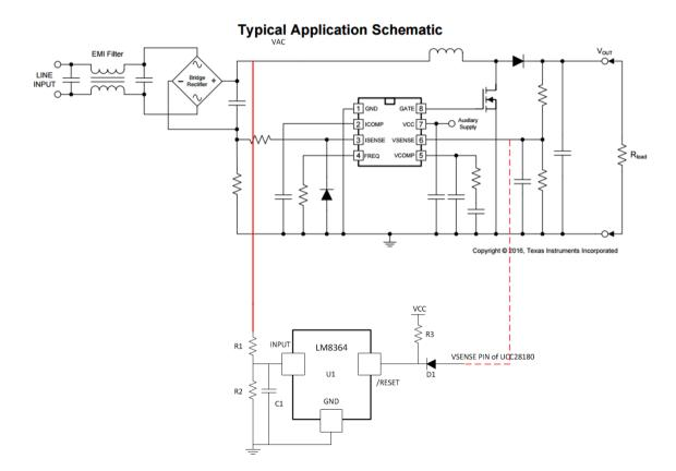
To apply brown out function with UCC28180, a external circuit with LM8364 is needed.
