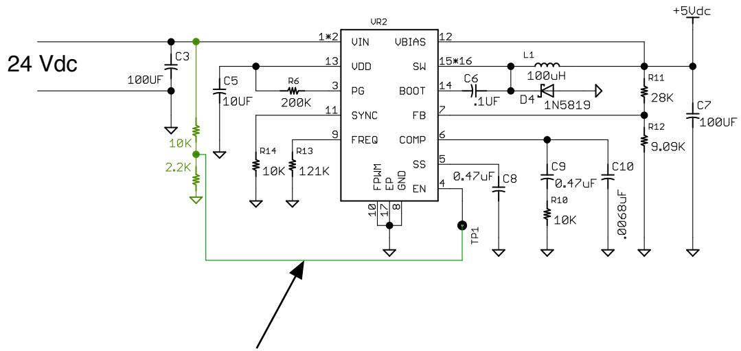
This is my fix for the voltage transient. It shuts off the 5v shortly before it begins to drop out, and seems to reset the soft start mechanism. I'm still curious about the transient though.
