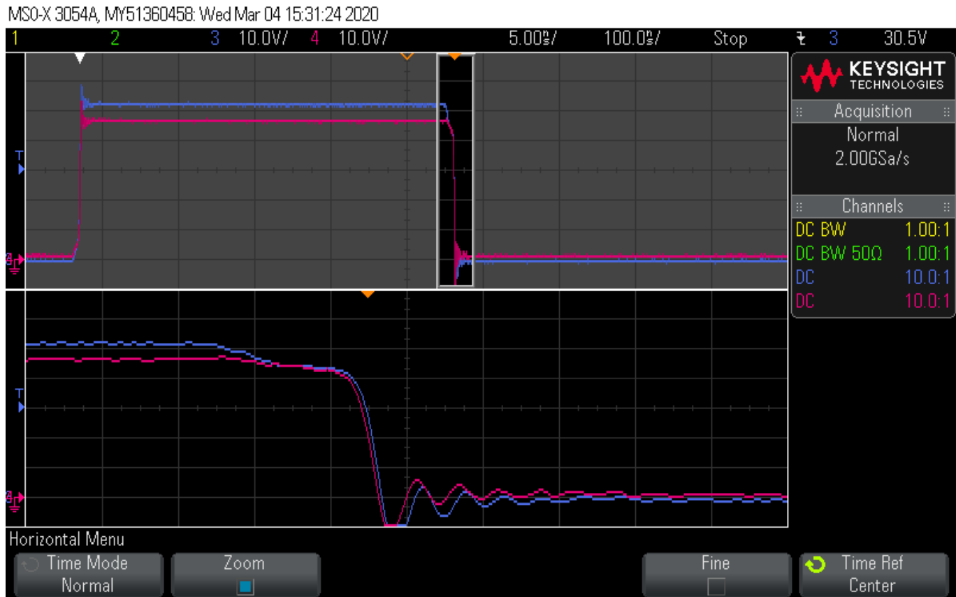
Figure 1 – LMGEVM_wL1 HO and HS during HS falling
