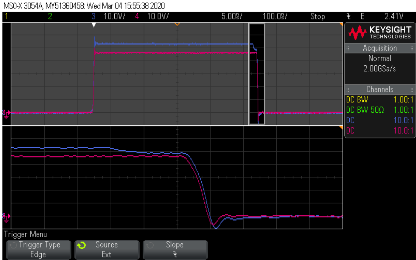
Figure 1 – LMGEVM_wL1 HO and HS during HS falling
