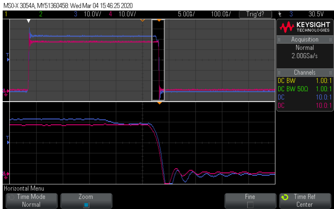
Figure 2 – LMGEVM_woL1 HO and HS during HS falling
