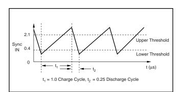
FIGURE 1. Internal Oscillator Timing.
