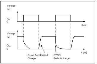
FIGURE 4. Emitter Follower Output Waveform V<sub>S</sub> and V<sub>IN</sub>
