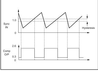
FIGURE 8. Comparator-Generated Timing Pulses.
