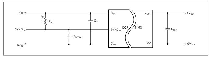
FIGURE 10. Connecting a Bleed Resistor.
