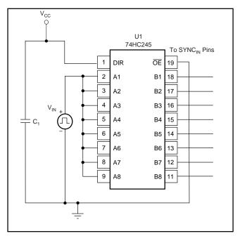
FIGURE 6. DCP01 Series HCMOS Interface.
