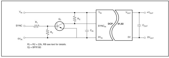
FIGURE 11. External Control of the DCP01, 02.
