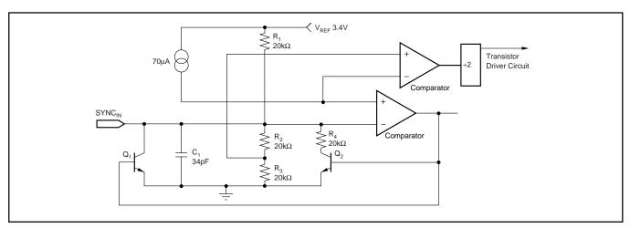
FIGURE 2. Internal Oscillator Circuit.
