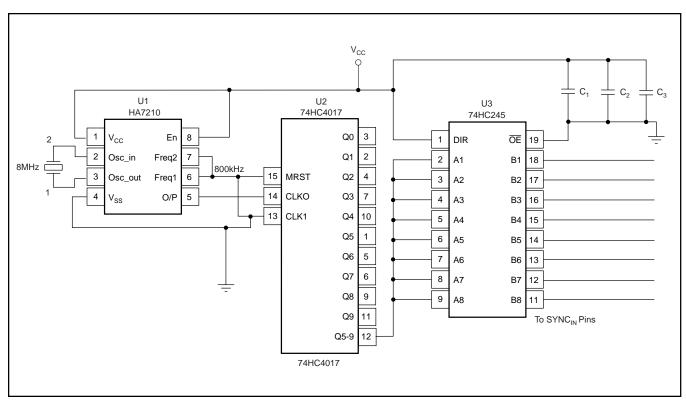
FIGURE 9. Crystal-Generated Clock Signal.
