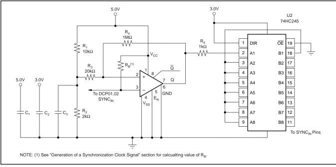
FIGURE 7. Comparator Generated Timing Pulses.
