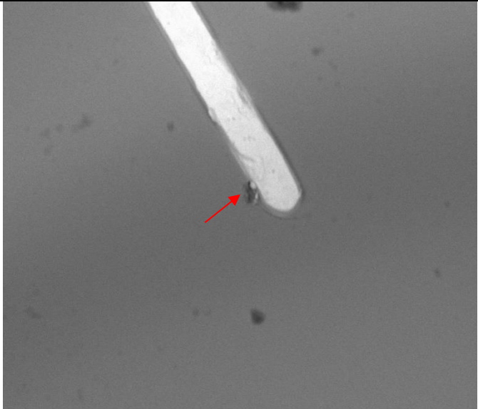
Fig 4f : Short Circuit LED: SEM closed up view observed blow hole on Die surface near metal trace
