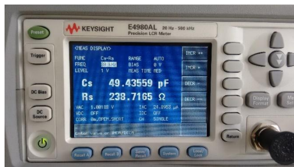
Fig. 3.25 Measurement of interwinding capacitance
