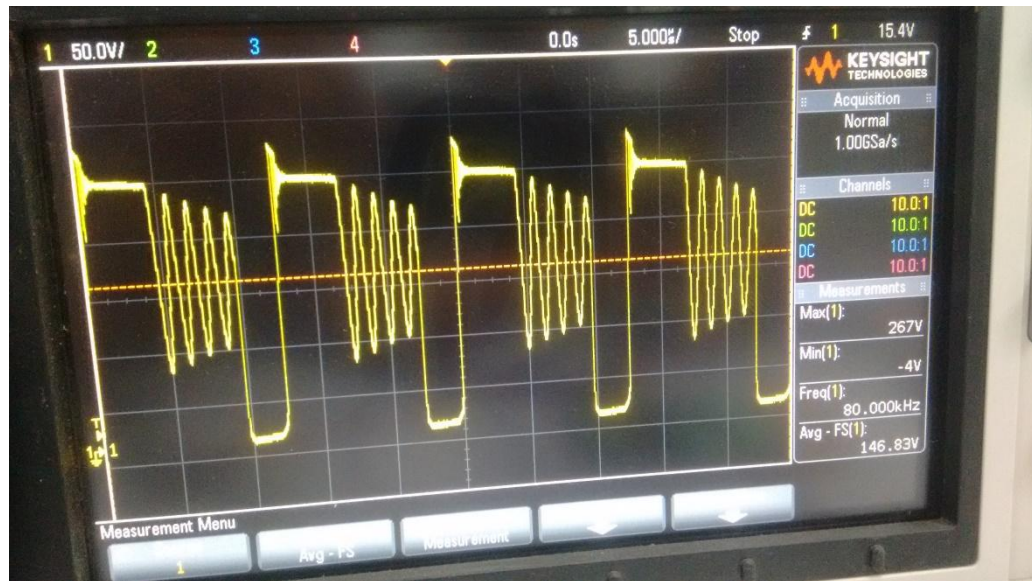
Fig. 5.8 Waveform at Drain and snubber
