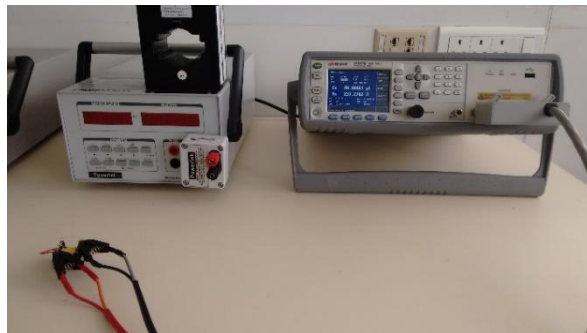
Fig. 3.24 Inter winding capacitance measurement test setup.
