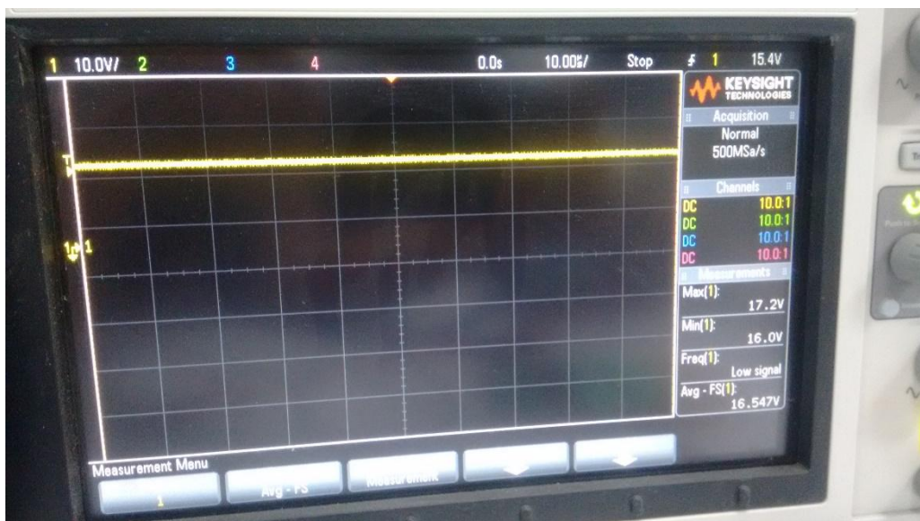
5.9 Waveform at supply pin of the IC
