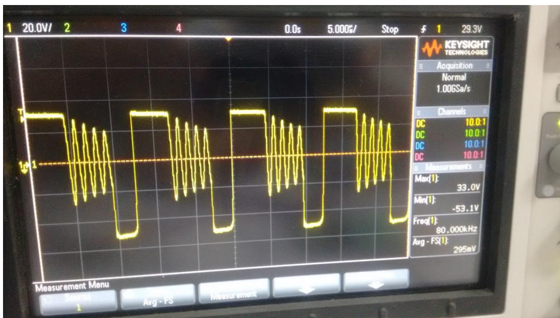
Fig. 5.10 Waveform at transformer pin 7
