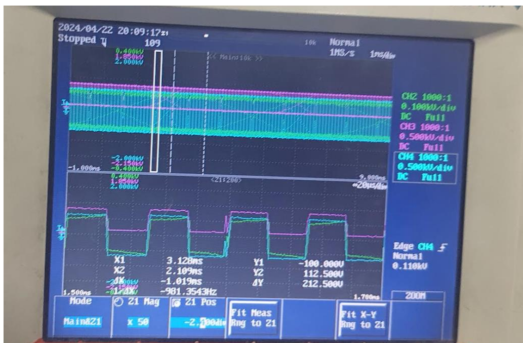
Figure 2: CH2: voltage across transformer, CH3: Voltage across MOSFET CH4: Voltage across MOSFET
