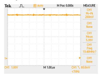
Below screenshot was taken at 6V with 6.9 $\Omega$  loads (870mA@6V) on each of the HEATER OUTPUTS. CH1 setup for AC voltage measurement.
