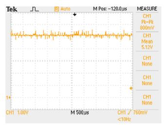
Below screenshot was taken at JX11 (Output of HEATER 1 BARRIER) with 6.9 $\Omega$  load (870mA@6V). CH1 setup for AC ripple measurement.
