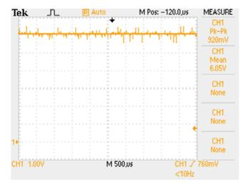
Below screenshot was taken across C12 (Output LMR16030) with 6.9 $\Omega$  load (870mA@6V). CH1 setup for AC ripple measurement.
