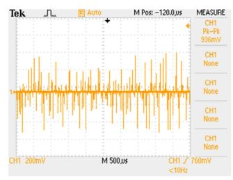
Below screenshot was taken across C12 (Output LMR16030) with 6.9 $\Omega$  load (870mA@6V). CH1 setup for DC voltage measurement.
