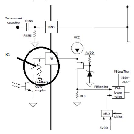
The FB pin has an internal current source that is used to control the oscillator frequency of 85.1 uA roughly. When the Opto transistor is off the IFB current is going through the internal RFB resistor and the controller is operating at the maximum switching frequency is at the maximum of 1 Mhz to reduce the LLC gain.
