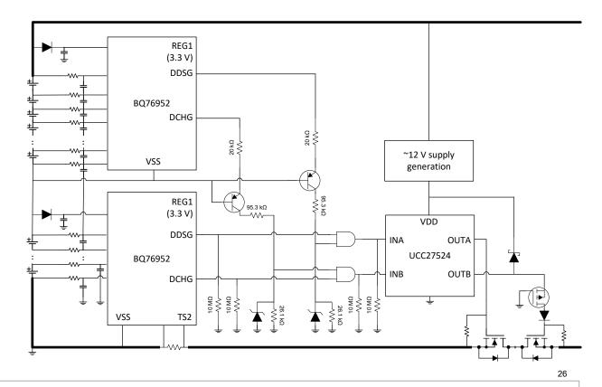
High cell count battery monitoring using BQ769x2
