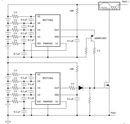
A simplified schematic of a 16S system using 4 stacked BQ7718 is shown
