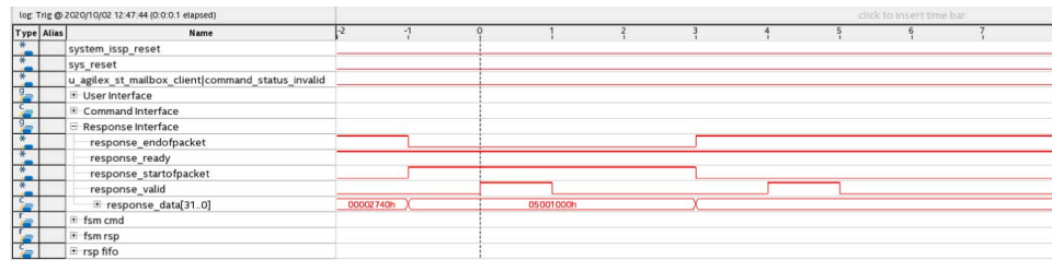
Figure 20. Signal Tap Capture of Response for GET_TEMPERATURE Command from the Mailbox Client with Avalon Streaming Interface IP
