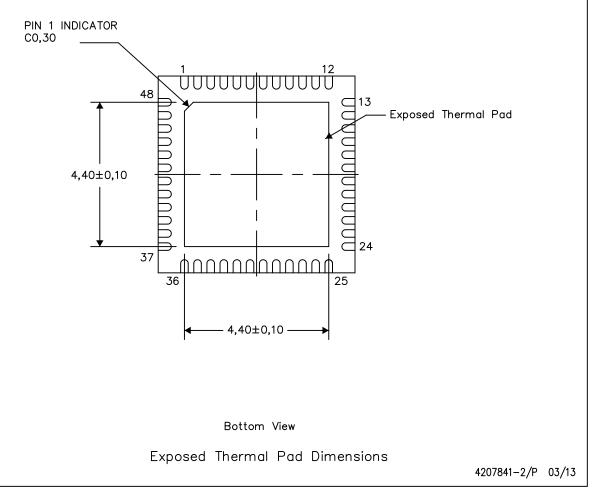
NOTE: All linear dimensions are in millimeters
