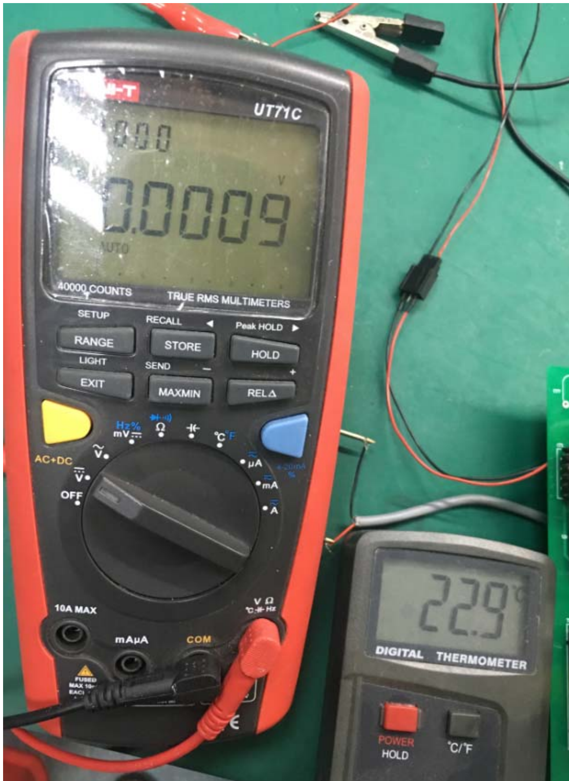
Fig3 Temperature measurement when IC Closed
