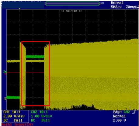
CH1:SW pin voltage CH2:EN pin voltage
