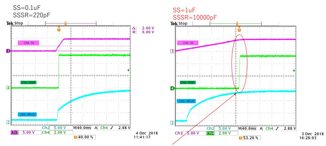
It should rise at 2 V, but it is rising at SS = 5 V. The difference is only the capacity value of SS and SSSR, but is there an upper limit of capacity value?
