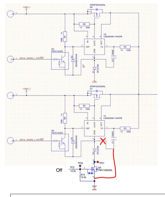
Can be repeated on top circuit.
