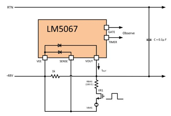
With the set-up above, the following data was collected. Note that it takes about 2mA of  $I_{OUT}$  current to make the gate go down. However it takes ~17mA to trigger an insertion delay.
