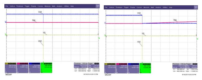
Once it was concluded that a VBIAS of 2.7V triggers an insertion delay, we zoomed in to find the corresponding VOUT and VR1 and t compute the IOUT.
