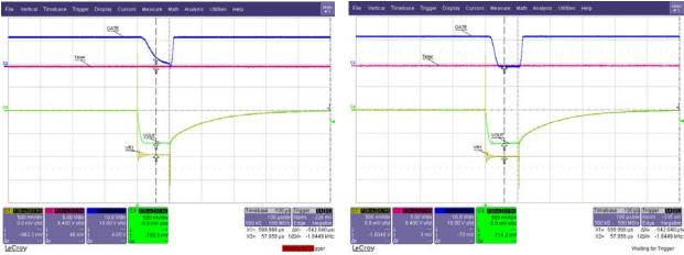
To find the threshold for triggering the insertion delay, VBIAS was raised until the insertion delay was observed. The left waveform was with a VBIAS of 2.65V and an insertion delay wasn't observed. The right waveform was with a VBIAS of 2.7V and an insertion delay was observed.
