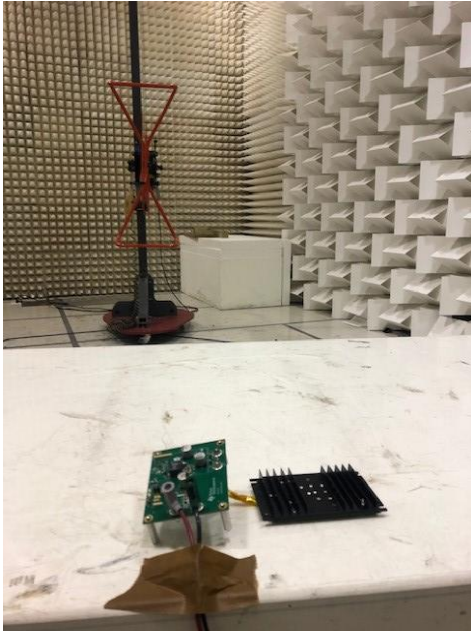
Figure 6-3 B Radiated Emissions Test Setup Back Heat Sink up, PCB Flat on Table
