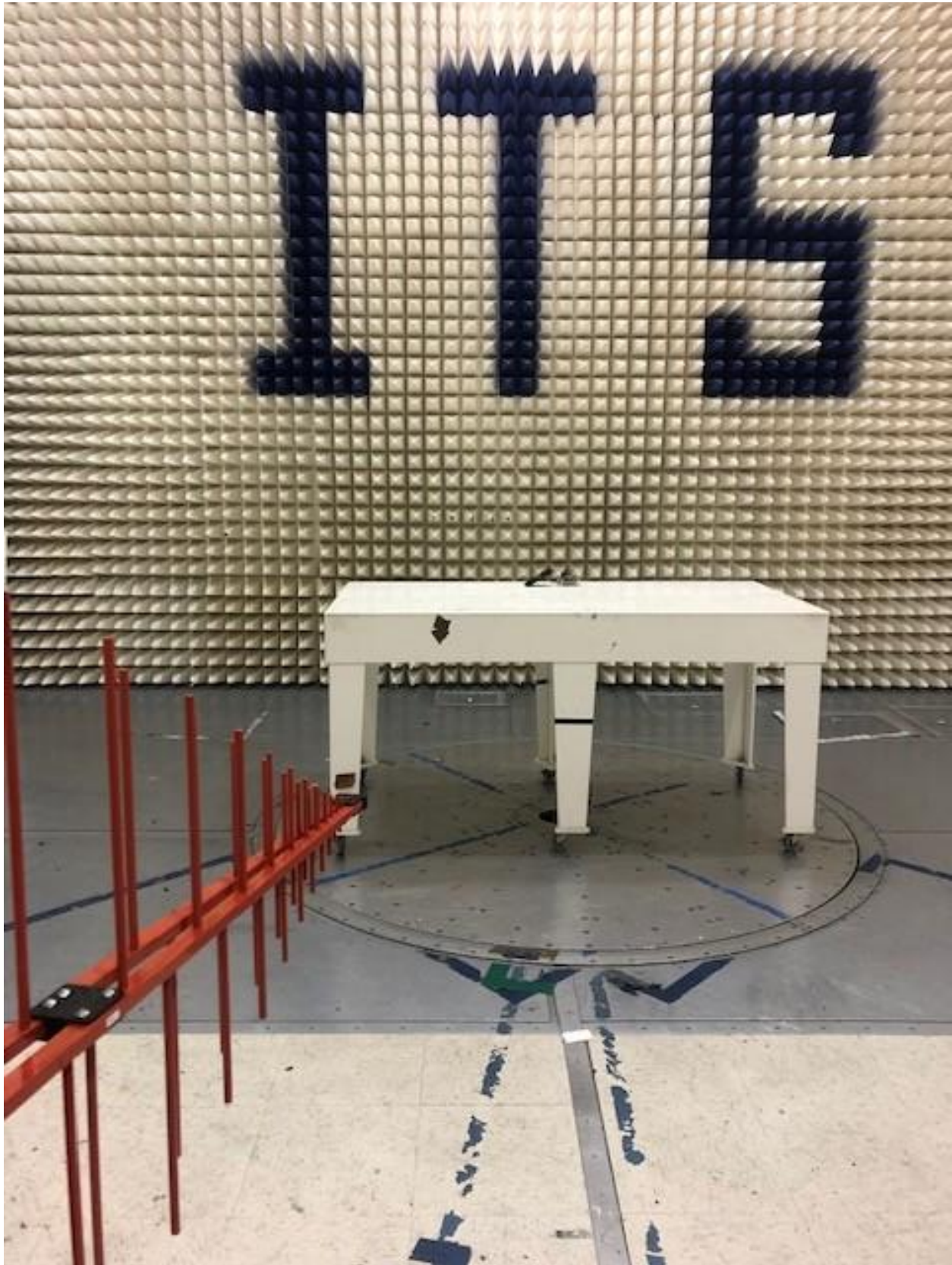
Figure 6-2 A Radiated Emissions Test Setup Front
