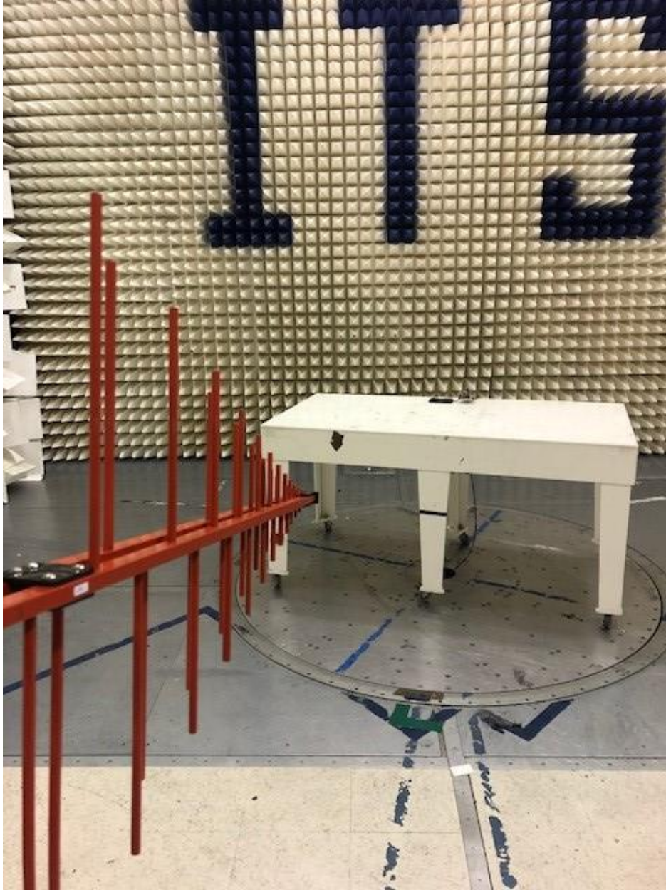
Figure 6-1 A Radiated Emissions Test Setup Front Heat Sink up, PCB Flat on Table
