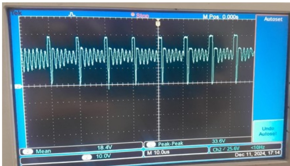
Fig6. Scope plot for H01 when input HV-PS=22V
