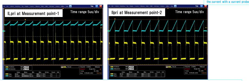
Even when the current waveform on the primary side is confirmed at measurement points 1 and 2 in the target condition of evm. the waveforms are different from each other the different current waveforms ware confirmed.
