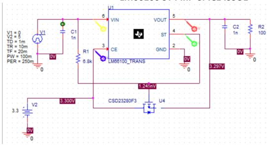
Simulation shows ST Pin never floats to +5v. Also, VOUT never goes to +5V because U4 MOSFET is still ON
