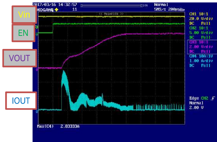
LMR14030SQDPR w/Spread Sepectrum T_{ss}=0.8\text{ms}
