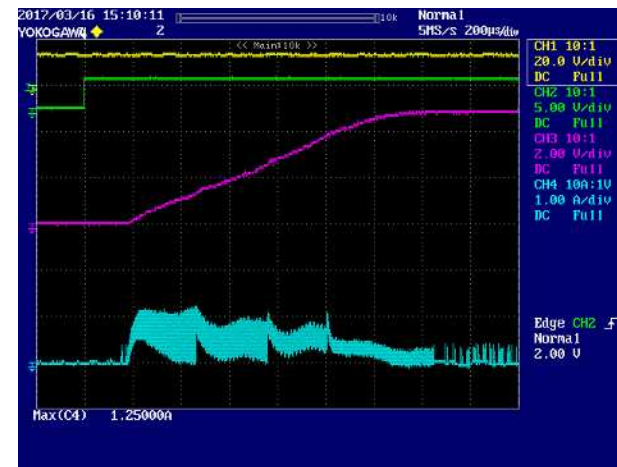
LMR14030QDPR w/o Spread Sepectrum T_{ss}=1.17\text{ms}
