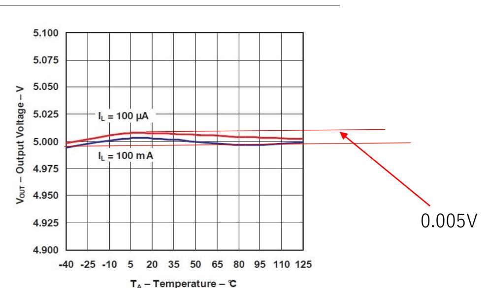
Figure 5. Output Voltage vs Temperature
