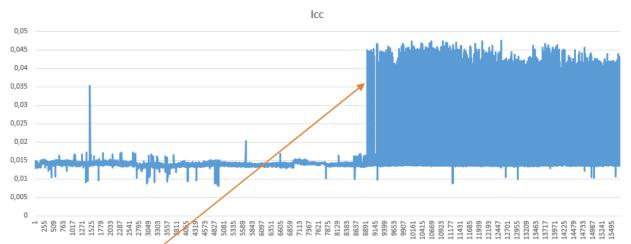
In this figure we see the input-current of approx. 15k Sensors, shown over time. At the 20<sup>th</sup> of February we have seen this failure with a current of approx. 40mA the first time. When we do an second run on the test system with the same sensor we often see a normal operation.
