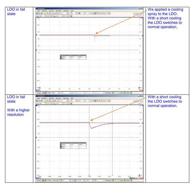
Then we have connected the On/OFF-Pin to an external Voltage of 5V. But this configuration shows the same bad results.
