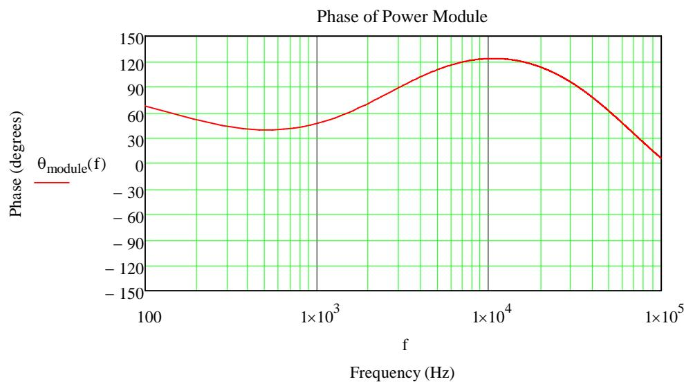
Want the total loop to cross at a decade or more before the module's crossover. To do this, determine what the gain of the module is at the desired system crossover frequency, determine the contribution from the open loop load share components, then select the error amplifier components to add the desired attenuation
