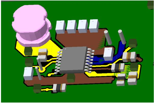
I've been trying to figure out editing the actual layout, adding more caps in the output (see image above), RC circuit in enable pin, etc. The actual image with that configuration is the closest one to achieve almost always -15v output. Also after some use, powering off and powering on again, won't come up to -15v but to +1V.
