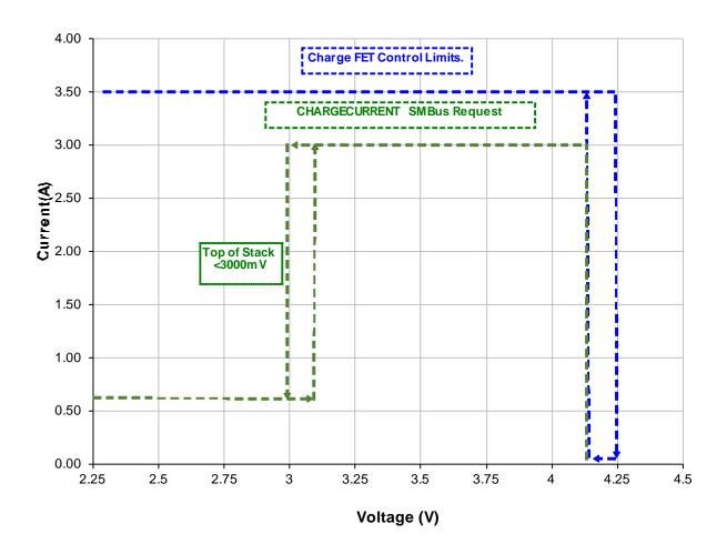
NOTE: The charging current requested from 3.0 to 4.2 V is defined by the temperature of the pack as shown in the preceding charge operating limits graph in this section. A 3.0A charge current is shown in this graph to represent the current defined by said graph.
