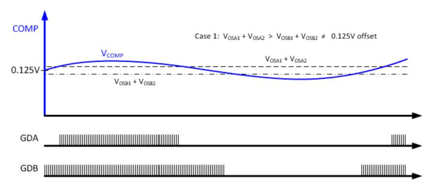
On-time of PWM:  $T_{ON} = K_T(COMP - 0.125V)$ Phase-A offsets are higher than Phase-B offsets. COMP is higher than Phase-B offsets more than Phase-A offsets, so Phase-B switches more than Phase-A.
