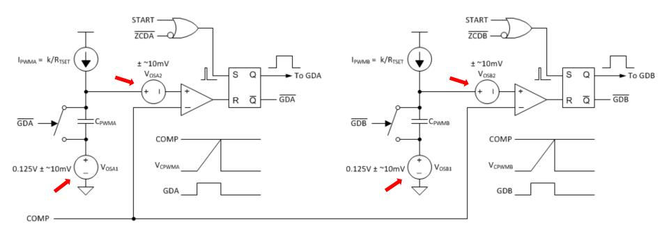
Phase-A and Phase-B have the same PWM generator circuits, but each has separate offset voltages at the ramp capacitor and the comparator.
