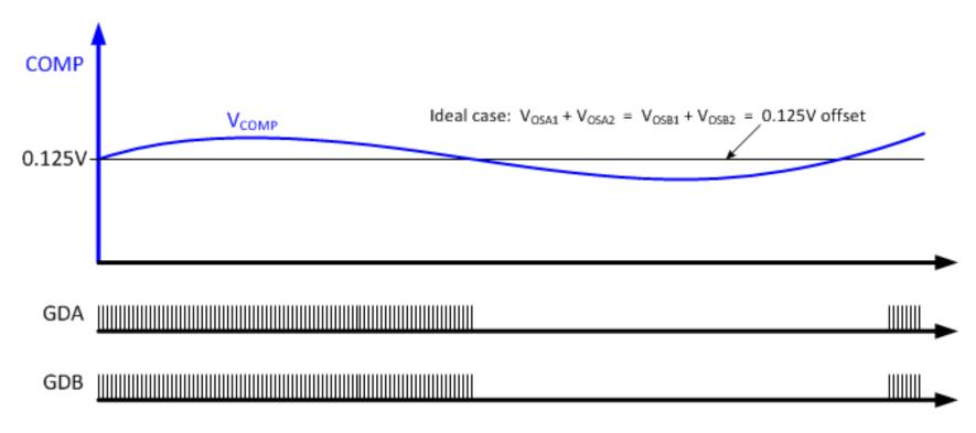
On-time of PWM:  $T_{ON} = K_T(COMP - 0.125V)$ Even at very light load, COMP has some ripple voltage on it. At high-line, COMP is very close to the 0.125V offset.
