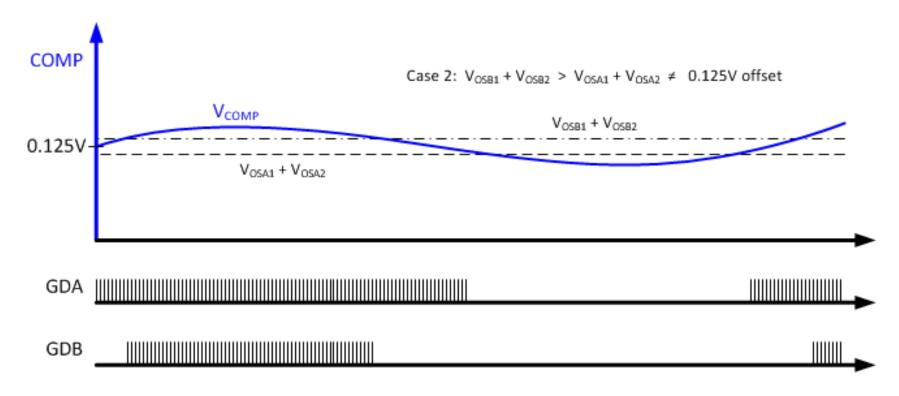
On-time of PWM:  $T_{ON} = K_T(COMP - 0.125V)$ Phase-B offsets are higher than Phase-A offsets. COMP is higher than Phase-A offsets more than Phase-B offsets, so Phase-A switches more than Phase-B.
