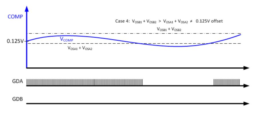
On-time of PWM:  $T_{ON} = K_T(COMP - 0.125V)$
