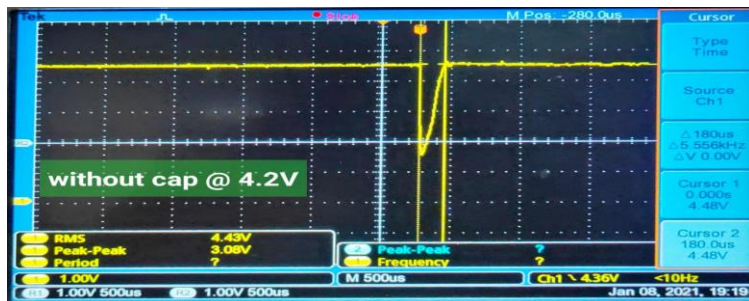
(Without 33uf cap at BAT Pin)
