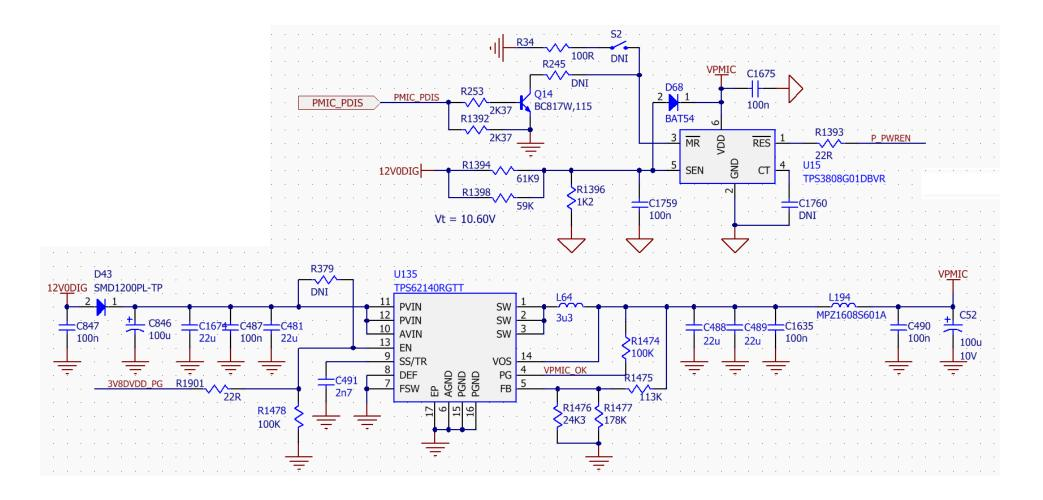
Here is the DCDC providing the Vin PMIC (VINDCDCx) ; VPMIC = +5.2V;
