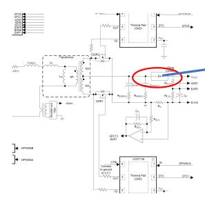
Or-ing diode kills the gains from sync rectification Is it there for "interleaving"?
