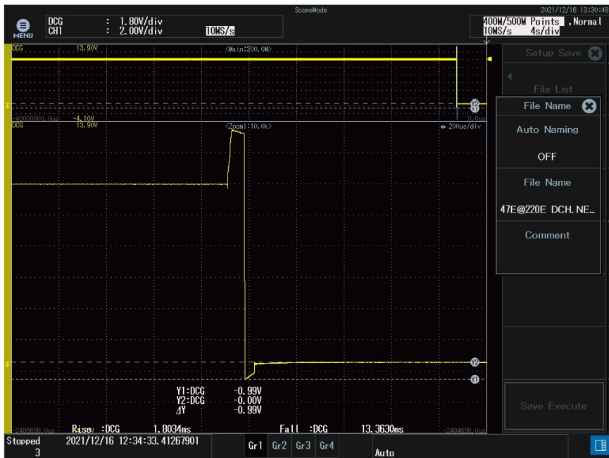
Mosfet gate discharge negative voltage Amplitude
