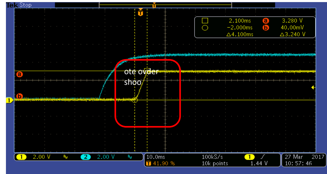
Fig#2. PTH05060W power-up with Track connected directly to 5Vin
