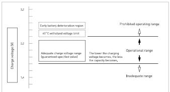
If the charge voltage goes beyond its adequate range, battery performance may deteriorate early. Be sure to observe the guaranteed charge voltage.
