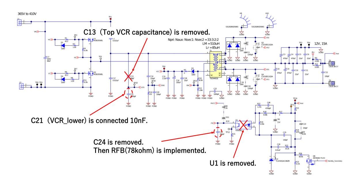
Figure 3. UCC25640EVM-020 Power Stage Schematic
